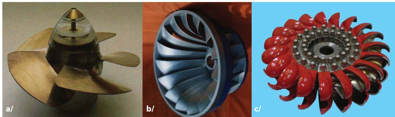
Obr. 4: Rotory vodních turbín (a/ Kaplanovy; b/ Francoisovy; c/ Peltonovy).
