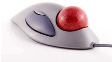
Since the whole device is not moved, a track ball requires less space than a mouse. A track ball comes in various shapes like a ball, a button and a square.
