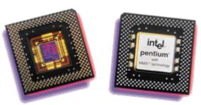
This generation can be characterized by both the jump to **monolithic integrated circuits(millions** of **transistors** put onto one integrated circuit chip) and the invention of the **microprocessor** (a single chip that could do all the processing of a full-scale computer). By
